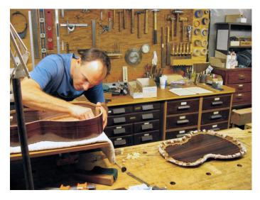
Each time that Joel made a change in the braces, or thickness of the top or back, we retaped the back onto the body, and ran a "response curve" with the computer. This allowed us to see the effect of what we had done, and track our progress.
