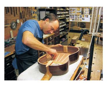
Shaving down the main back brace across the lower bout has most of it's effect on the frequency of the air resonance.
