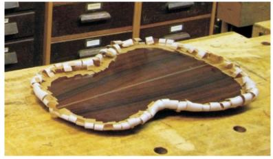
his first guitar, a "larger model" classical with East Indian Rosewood back and sides, and an LS redwood soundboard. To the left is the back that has been removed from the body to give him access to the braces for doing the "final voicing". The braces are purposely installed a little taller than necessary to allow for trimming.
