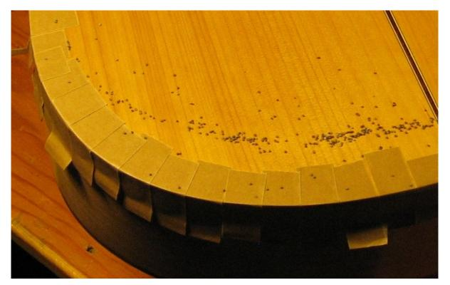
Taping on of back. To remove it from the body, it is only necessary to lift the tabs until the tape is just stuck to the back.
